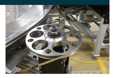
The belt was implemented in the table's design (similar applications exist) and is tensioned with the small roller. The majority of the belt is in contact with the rotating table.
